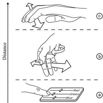
**Figure 1:** In this example, a user can pick the color of a moodlight at varying levels of control. It enables (a) fine control via touch on the device, (b) in-air control of brightness and hue by moving and rotating the hand, and (c) abstract control of mood by waving over the device.
