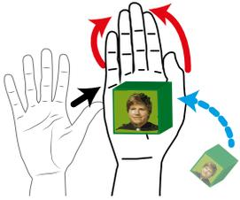
**Figure 4:** Object selection (top) and pick-up of objects by moving the fingers of the hand together (bottom).
