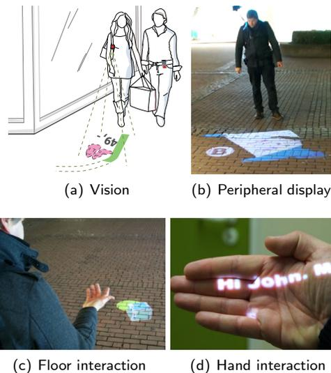
**Figure 1:** (a). The vision: a wearable peripheral display (e.g., on the floor). (b) A user serendipitously discovers information. (c) The user has received a text message and picks it up from the floor. (d) The scrolling message text is read in the user's hand.
